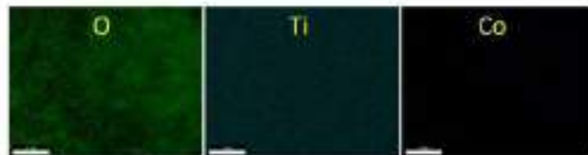
Figure S1. EDS maps of the O, Ti and Co distributions.
