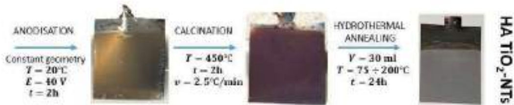
Figure 9. Schematic of the synthesis of HA TiO 2 -NTs via anodisation, calcination, and hydrothermal annealing.
